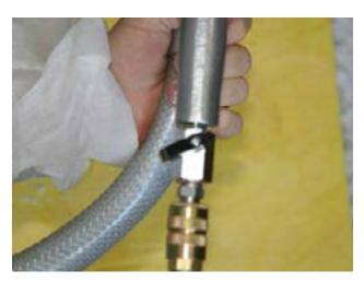
Adjust the air flow valve as needed.
