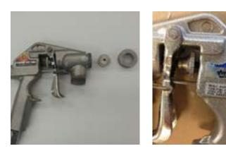
For the EB2 finish coat use size 3 orifice with the smallest outer fan tip (A). The material flow would normally be set to the 4th ascending dot for fine texture and 5th ascending dot for medium texture. The air vent is fully open and the material flow control on the spray gun (see picture) is set to be almost closed. (When it is in accurate position you will only get a spray mist, without any splattering.)
