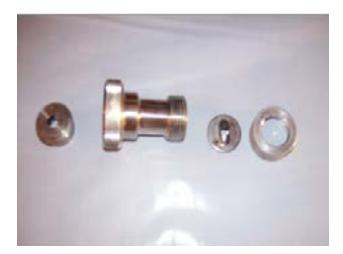
For the Silk finish use size 6 orifice with the second largest outer fan spray tip (C) near right. The material flow on the Graco RTX 1500 would typically be set to the 3rd ascending dot.
