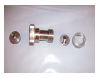
For the EB1 finish coat use #8 orifice with the second largest outer fan spray tip (C) near right. You may need to adjust the components to match the desired texture. Some applicators prefer not to use the fine finish kit when creating a Natural finish the golden rule is to match the mock-up.
