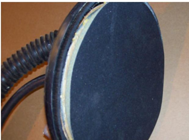
Remove the bristle guard from the vacuum sander so that the bristles do not restrict any sanding to the surfaces and prevents damage to the board and basecoat layers.
