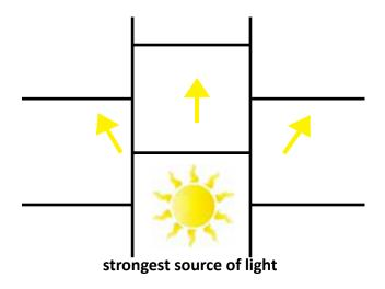
Wherever possible install the Fellert acoustical boards so the longest runs of joint lines flow into and away from the strongest source of light. This process is deemed a "best practice" only and not an absolute rule. It is a simple and a logical approach to help minimize any shadowing effects which can be exacerbate by critical lighting.
