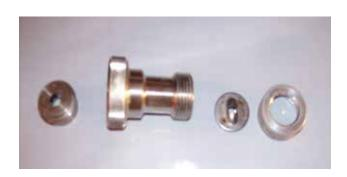
For the Silk (Even Better 2) top coat use size 6 orifice with fan spray tip (8-12) near right. The material flow on the Graco RTX 5000 PI would typically be set to the 3rd-4th ascending dot.
