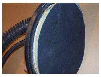
Remove the bristle guard from the vacuum sander so that the bristles do not restrict any sanding to the surfaces and prevents damage to the board and basecoat layers.
