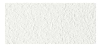
Spray consistently and eliminate spattering on plaster surface leave to dry 1-2 days. Dry thickness of the plaster finish will be approximately 3 mm (1/8").
