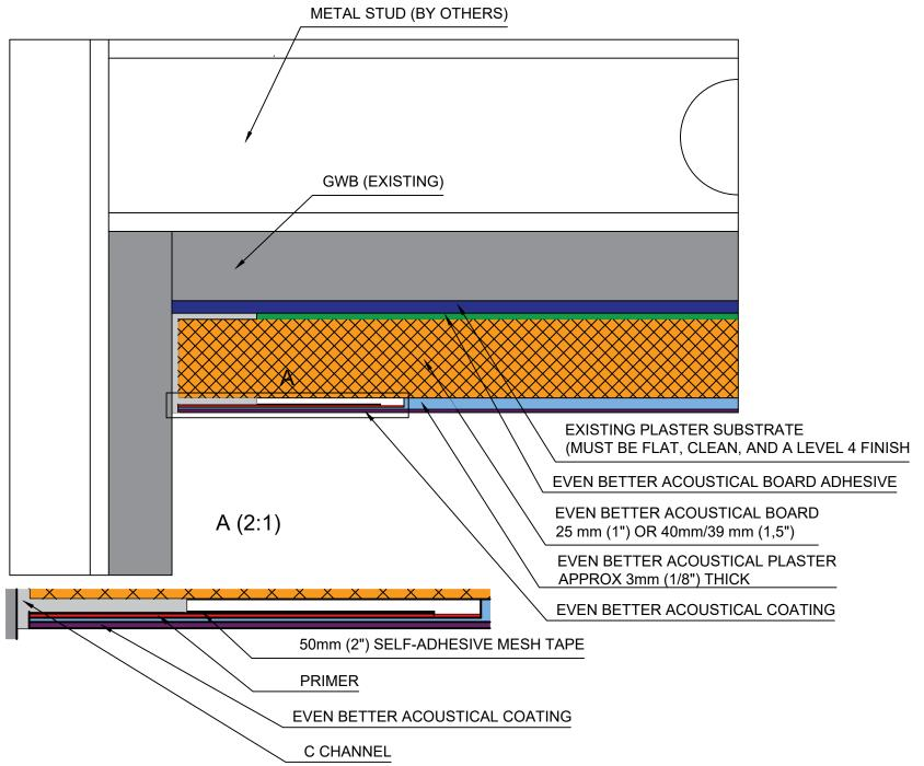
NOTE: ADDITIONAL MACHANICAL FASTENERS MAY BE USED IN CONJUNKTION WITH ADHESIVE
